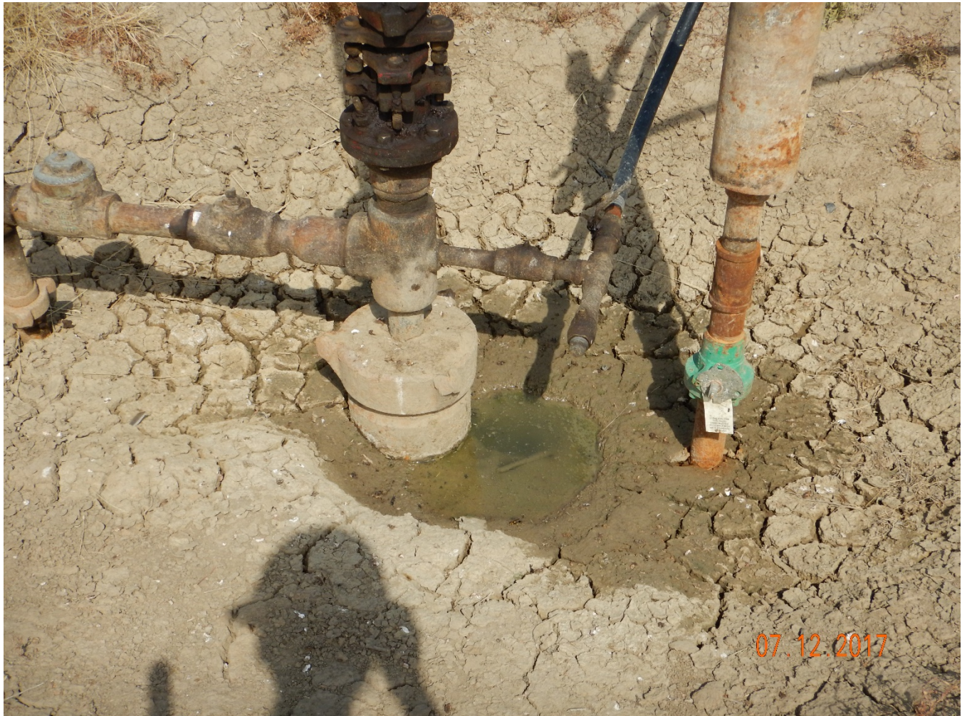
Figure 3 - Puddle surrounding wellhead. A steady release of bubbles into puddle was observed at wellhead, indicating possible integrity issue. An audible gas leak was also observed coming from 1" line on east side of wellhead.
