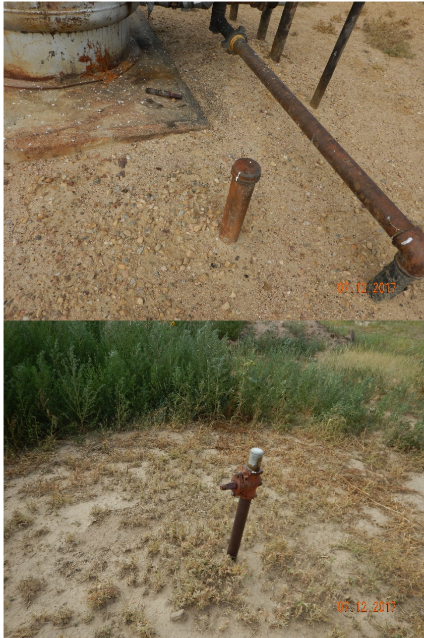
Figure 13 - Abandoned flowline risers at heater treater (top) and south of heater treater (bottom) had not been marked or tagged to comply with 2017 Flowline NTO as of inspection date.
