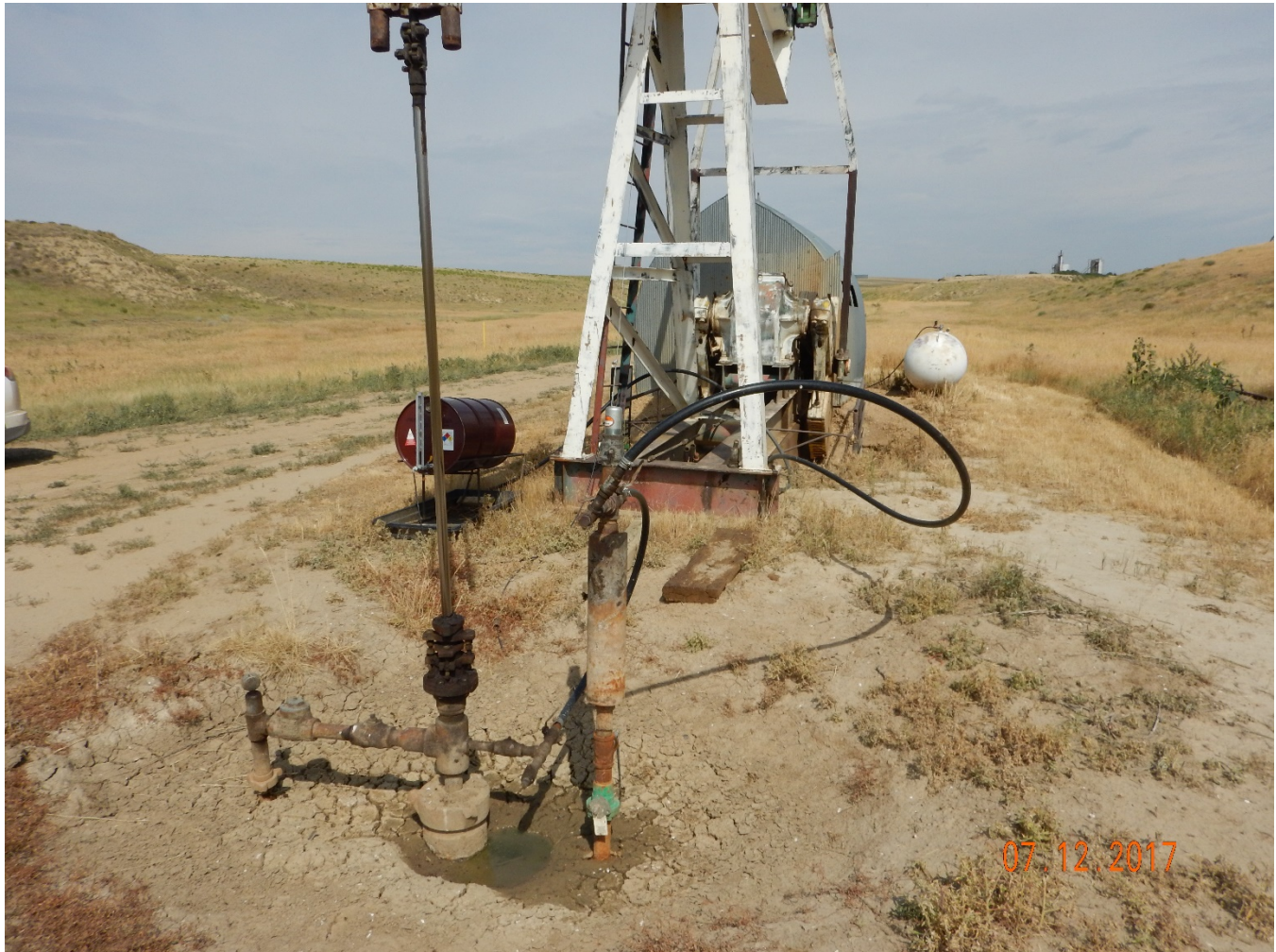
Figure 2 - Wellhead, pumping unit, 55-gallon storage drum, and propane tank. Note: wellhead remains surrounded by water.
