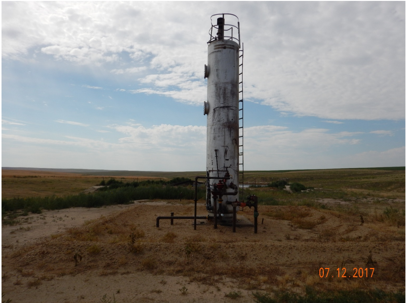
Figure 12 - Vertical heater treater with earthen berm and adequate bird protection.
