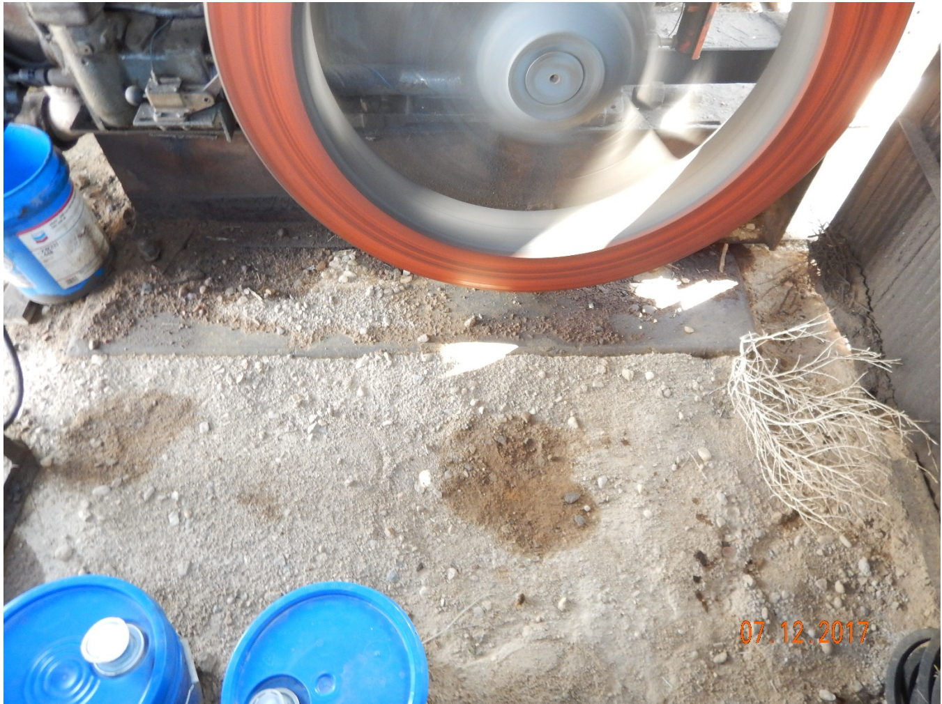
Figure 5 - Lube oil staining observed at prime mover.
