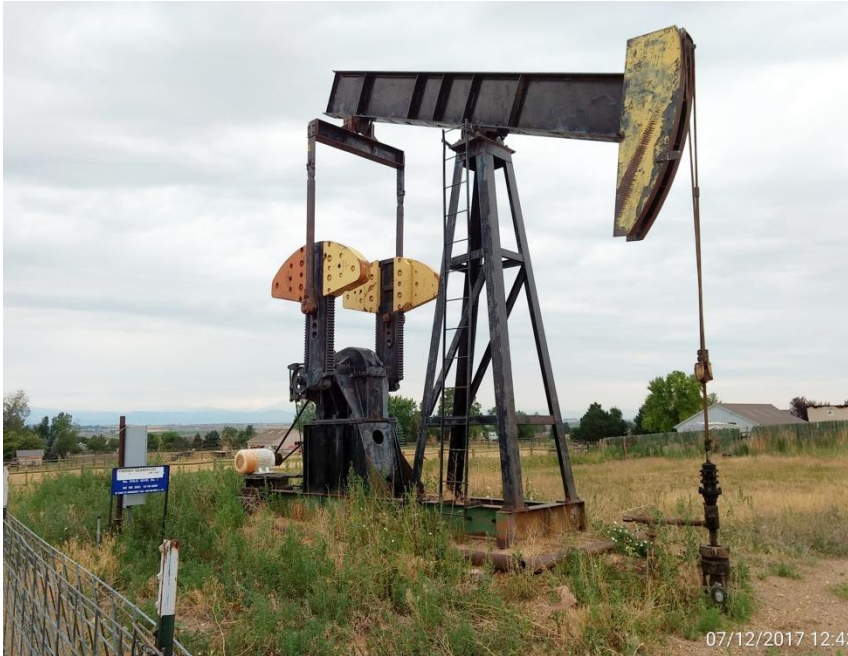
Wellhead and conventional pumping unit. Corrective Action: signage has inaccurate emergency contact info, overgrown weeds.
