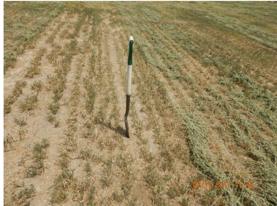
Photo 3: Photo taken from the adjacent reference area. Photo shows inspector had little resistance penetrating the topsoil in the reference area.
