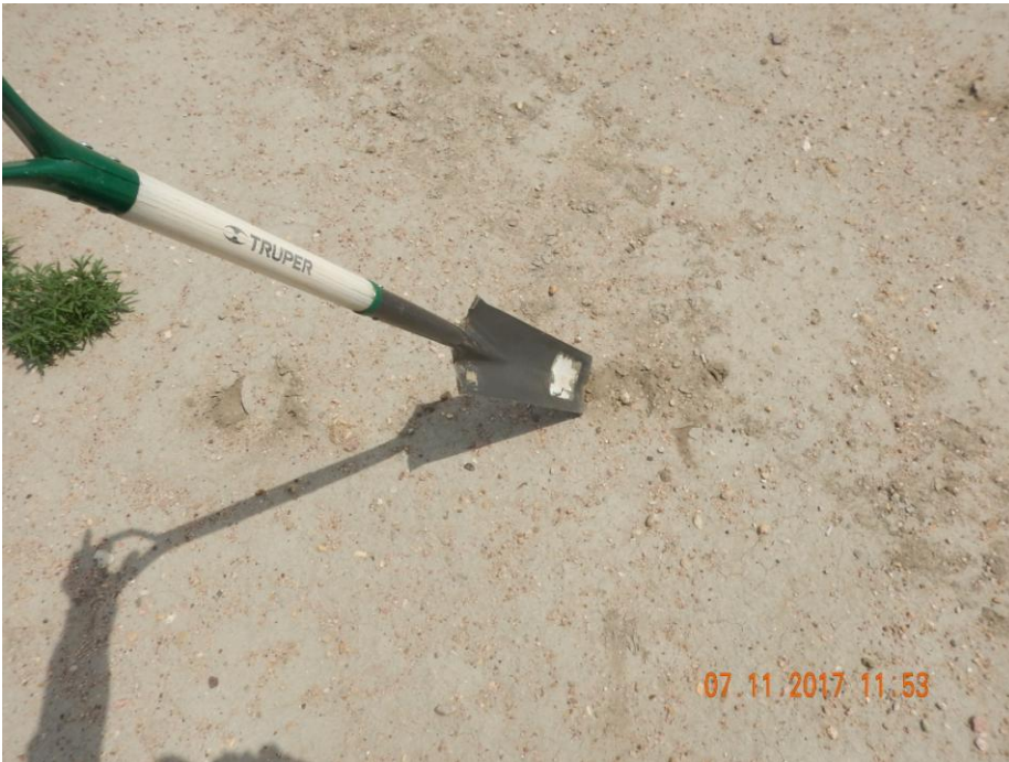
Photo 2: Photo taken from the battery location. Inspector attempted to dig multiple soil pits to test for compaction. Photo shows inspector was unable to penetrate more than ½ an inch throughout battery location. Compaction alleviation has not been sufficiently performed.
