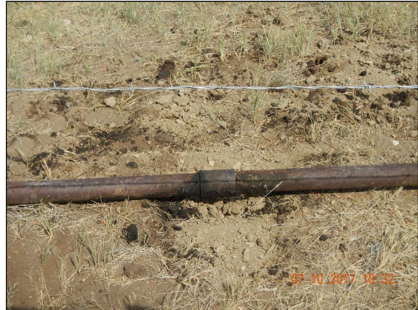
Photo 6. Close-up of leak and clean-up efforts at threads.
