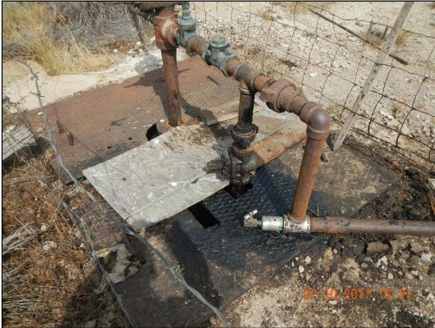
Photo 1. Wellhead with no fluid in cellar.
