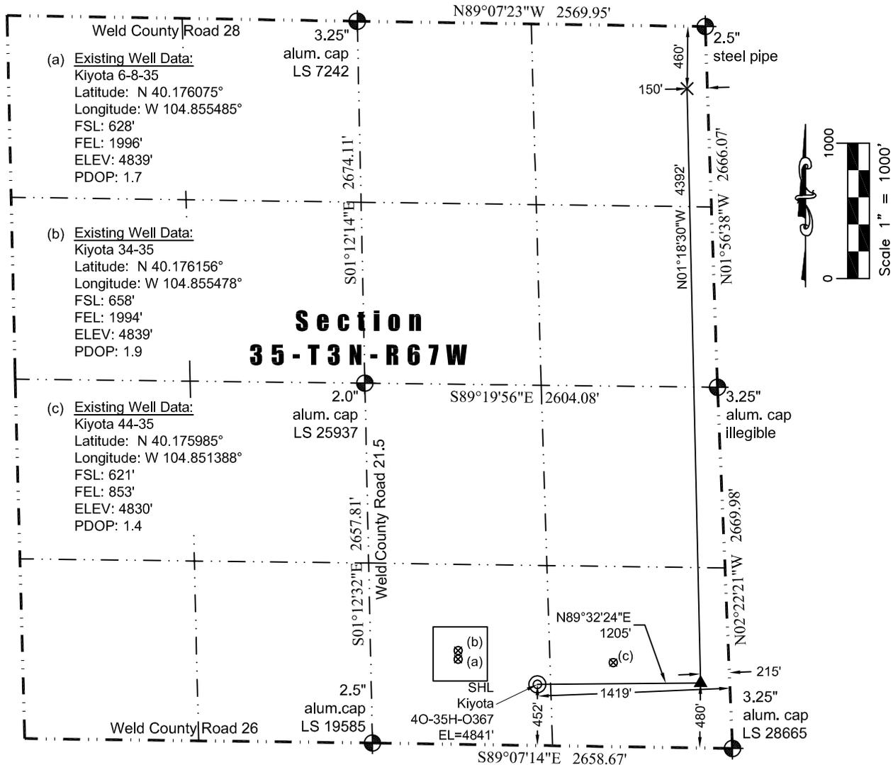
In accordance with a request from Jay Knutson of Crestone Peak Resources, Washburn Land Surveying, LLC has determined the location of the **Kiyota 40-35H-O367** well site to be SHL: 452' FSL and 1419' FEL, (TPZ: 480' FSL and 215' FEL), (BHL: 460' FNL and 150' FEL), as measured at ninety (90) degrees from the section lines of Section 35, Township 3 North, Range 67 West of the 6th Principal Meridian, Weld County Colorado.
