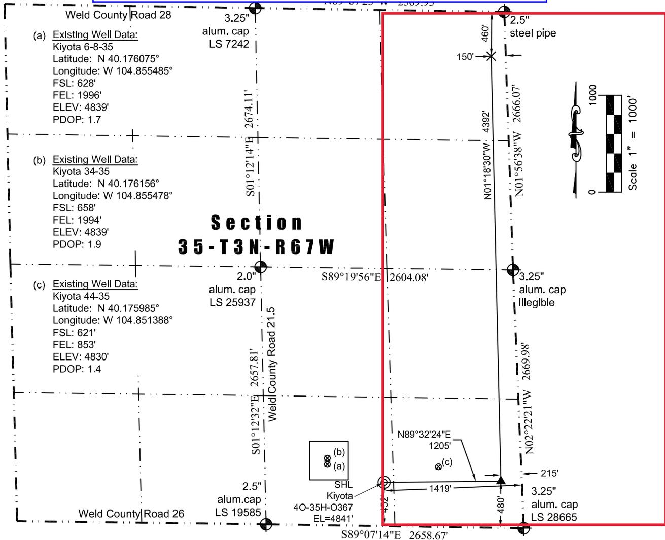
In accordance with a request from Jay Knutson of Crestone Peak Resources, Washburn Land Surveying, LLC has determined the location of the **Kiyota 40-35H-0367** well site to be SHL: 452' FSL and 1419' FEL, (TPZ: 480' FSL and 215' FEL), (BHL: 460' FNL and 150' FEL), as measured at ninety (90) degrees from the section lines of Section 35, Township 3 North, Range 67 West of the 6th Principal Meridian, Weld County Colorado.
