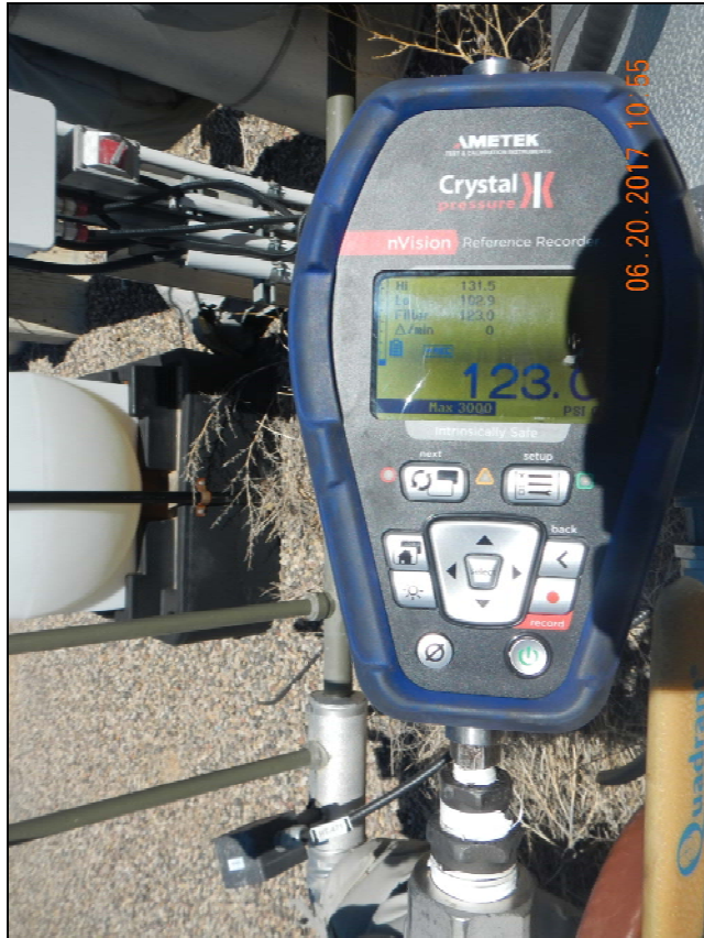
Photo 1. Gauge at beginning of test. 123.0 psi.
