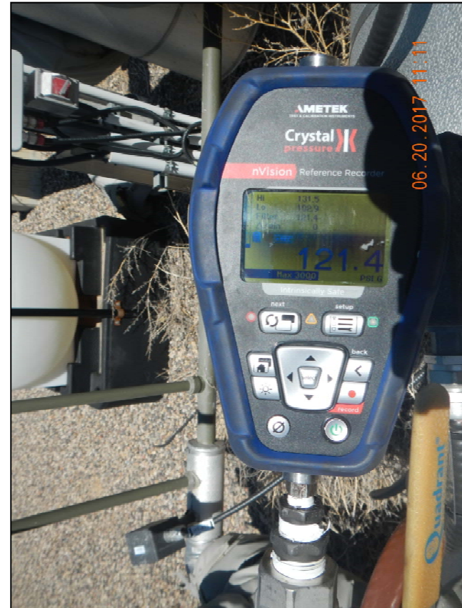
Photo 2. Gauge after 15 minute test. 121.4 psi.
