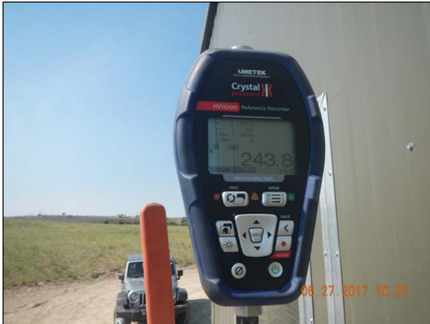
Photo 1. Gauge at beginning of test. 243.9 psi.
