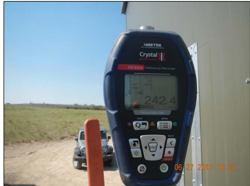
Photo 2. Gauge after 15 minute test. 242.4 psi.
