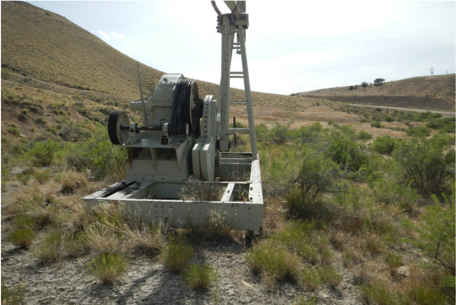
Photo#10: Pump Jack on Location..
