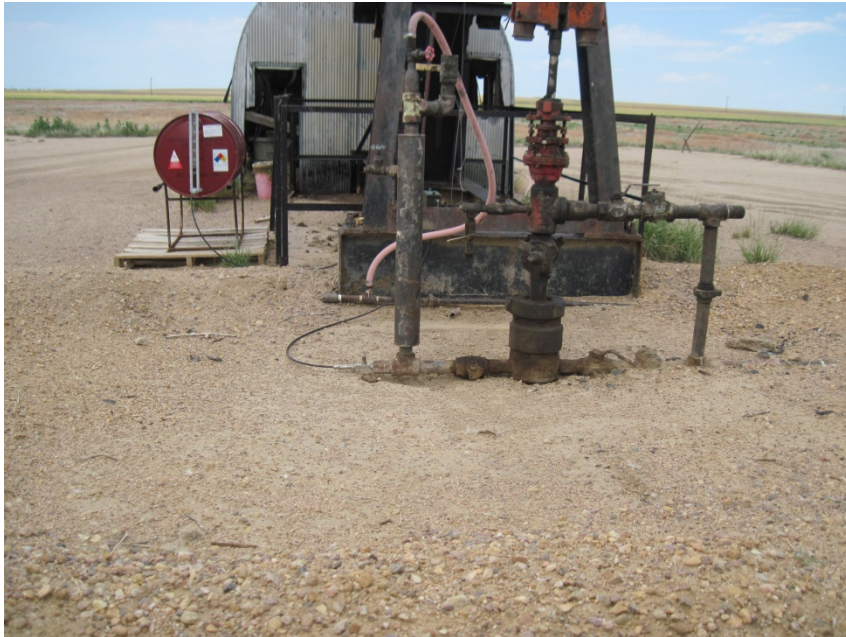
WELL HEAD NEED BRADENHEAD PLUMBED TO SURFACE
