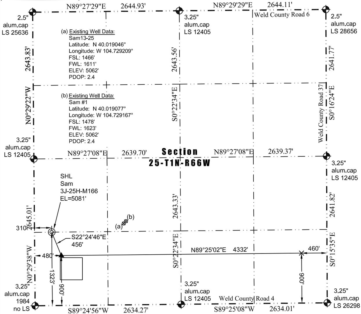
In accordance with a request from Jay Knutson of Crestone Peak Resources, Washburn Land Surveying, LLC has determined the location of the **Sam 3J-25H-M166** well site to be SHL: 1323' FSL and 310' FWL, (TPZ: 900' FSL and 480' FWL), (BHL: 900' FSL and 460' FEL), as measured at ninety (90) degrees from the section lines of Section 25 Township 1 North, Range 66 West of the 6th Principal Meridian, Weld County Colorado.
