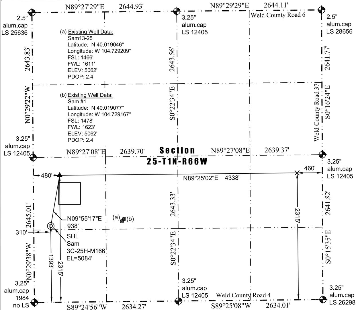
In accordance with a request from Jay Knutson of Crestone Peak Resources, Washburn Land Surveying, LLC has determined the location of the **Sam 3C-25H-M166** well site to be SHL: 1393' FSL and 310' FWL, (TPZ: 2315' FSL and 480' FWL), (BHL: 2315' FSL and 460' FEL), as measured at ninety (90) degrees from the section lines of Section 25 Township 1 North, Range 66 West of the 6th Principal Meridian, Weld County Colorado.
