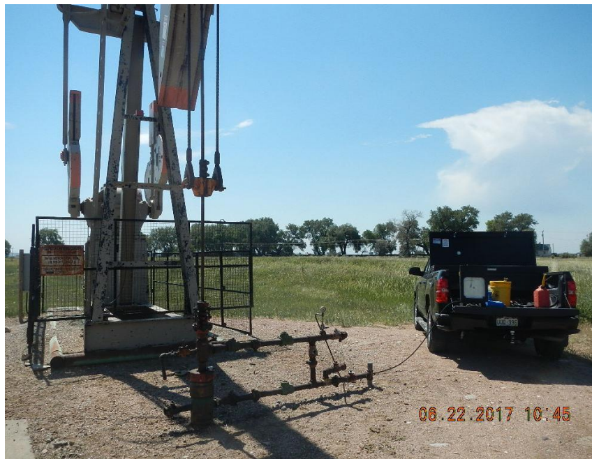
Photo 1 Wellhead with chart connected to flowline from west
