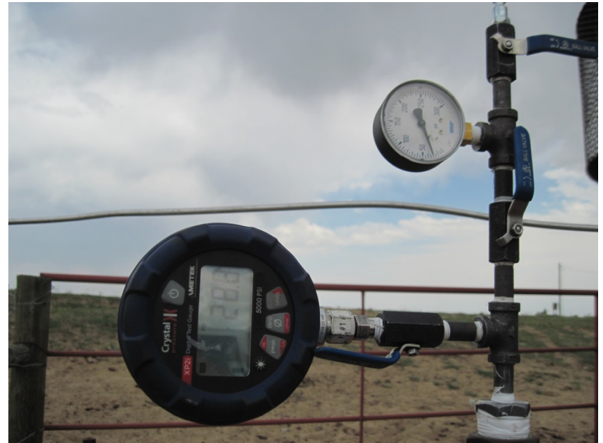
PRESSURE GAUGE AND RECORDER ECD 3" GAS LINE FROM OIL PROD TANK
