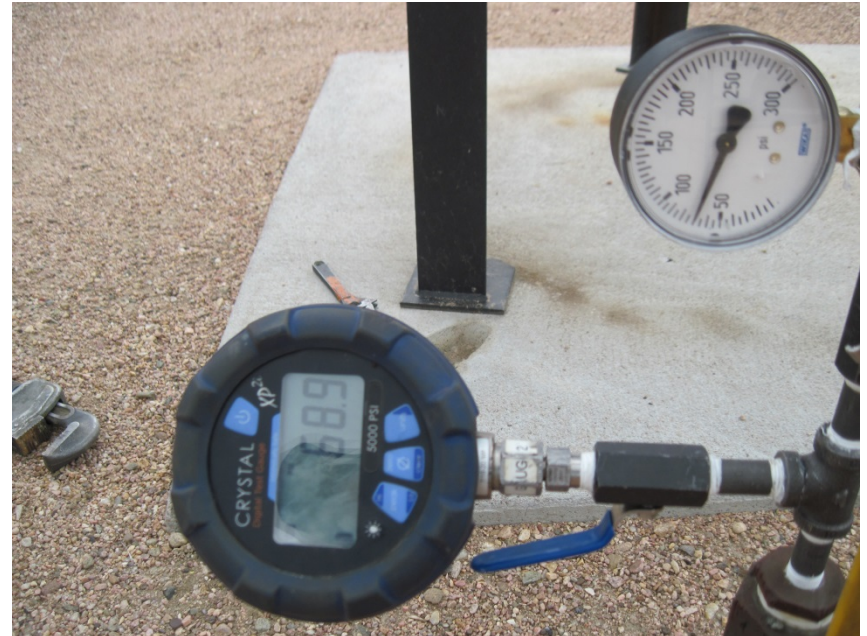
PRESSURE GAUGE AND RECORDER ECD 1" GAS LINE FROM SEPERATOR
