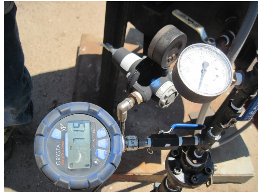
PRESSURE GAUGE AND RECORDER ECD 2" BLOW DOWN LINE FROM OIL PROD TANK
