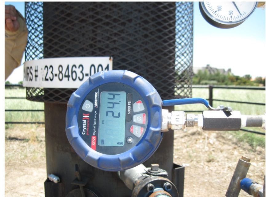
PRESSURE GAUGE AND RECORDER ECD 1" GAS SUPPLY LINE FROM OIL PROD TANK LINE
