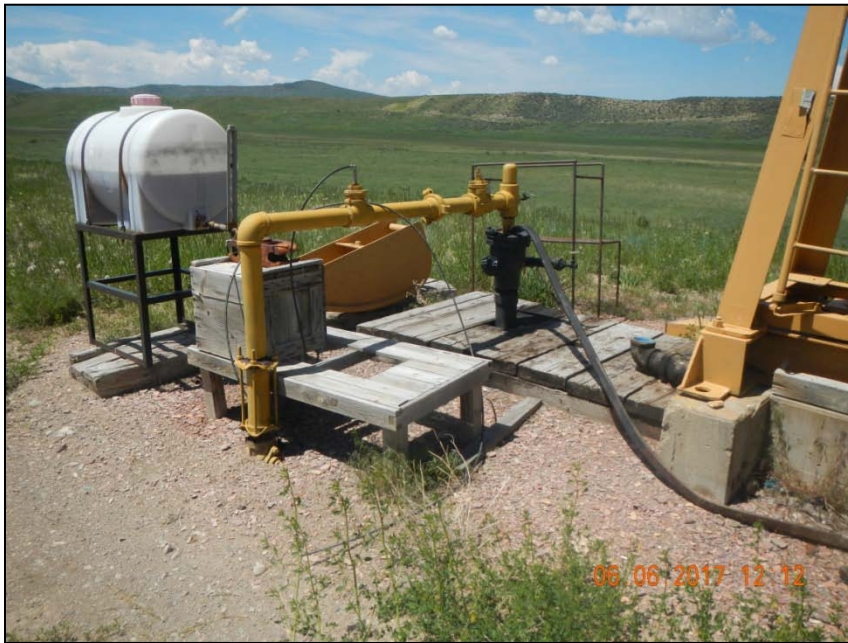
Photo 2. Risers at wellhead. No wellhead sign.
