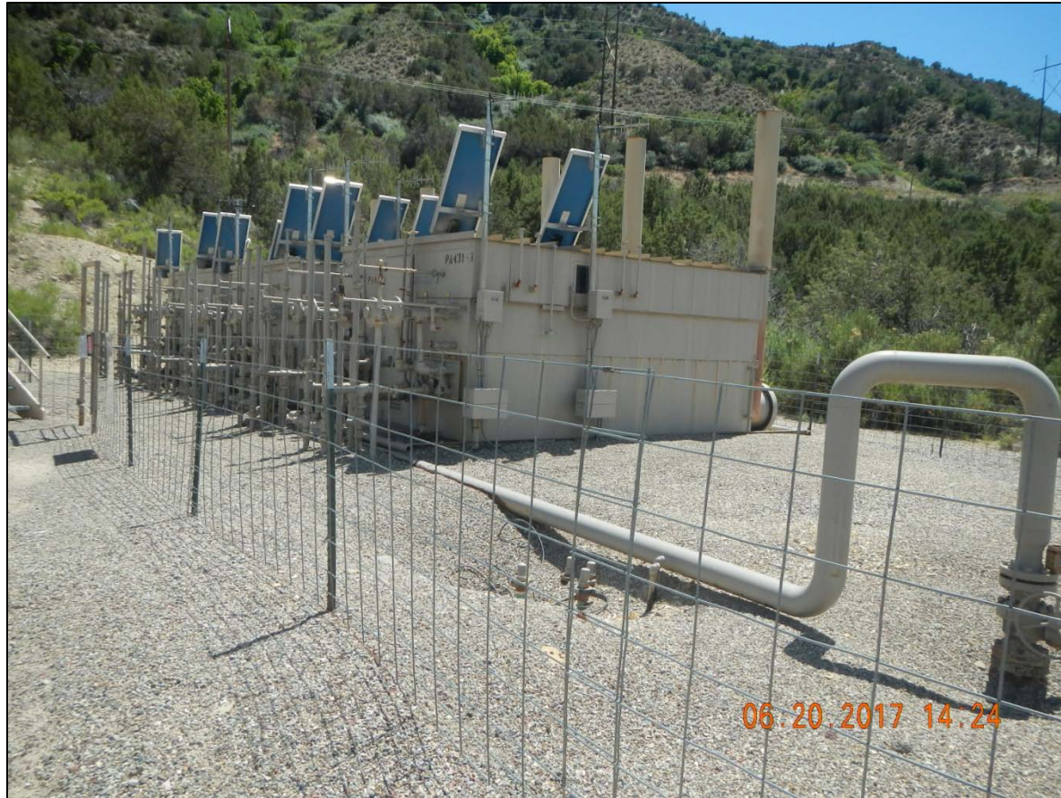
Unused risers by separators
