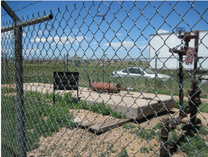
WELLHEAD SIGN AND SCRUBBER
