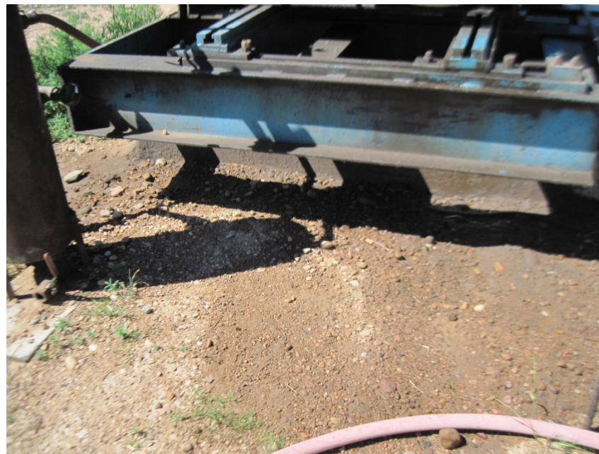
STAINED SOIL AROUND MOTOR MOUNTS
