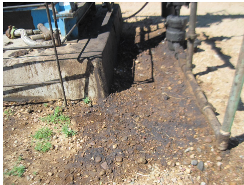
STAINED SOIL AROUND WELLHEAD
