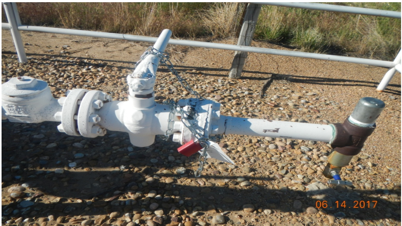
photo 4: There valve is locked out however the tagged is faded and cannot be identified.
