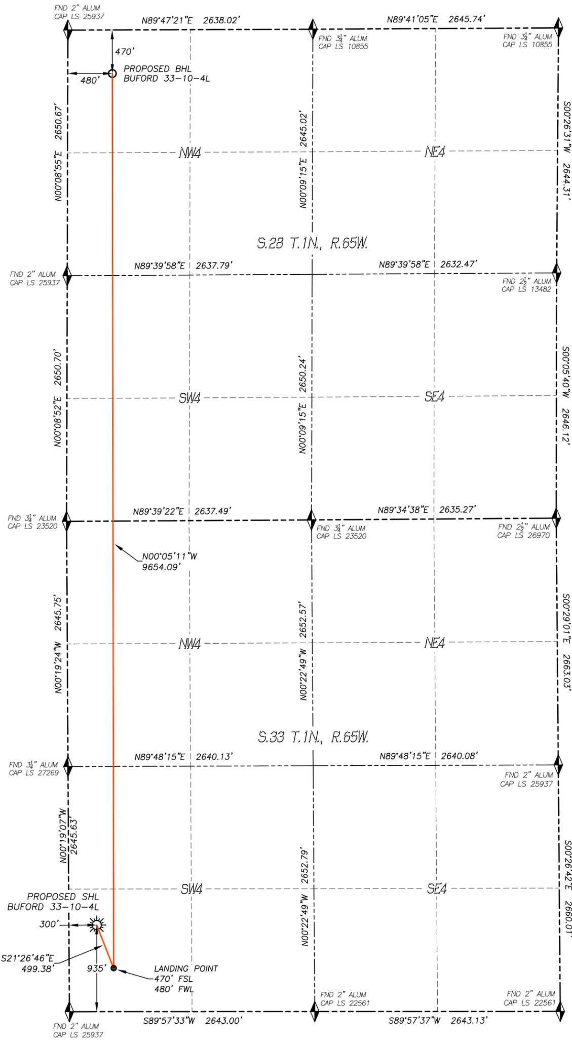
IN ACCORDANCE WITH A REQUEST FROM CONFLUENCE RESOURCES, DALEY LAND SURVEYING, INC. HAS DETERMINED THE SURFACE LOCATION OF THE BUFORD 33-10-4L WELL TO BE 935' FSL, 300' FWL, AS MEASURED AT NINETY (90) DEGREES FROM THE SECTION LINES OF SECTION 33, TOWNSHIP 1 NORTH, RANGE 65 WEST AND THE BOTTOM HOLE LOCATION TO BE 470' FNL, 480' FWL, AS MEASURED AT NINETY (90) DEGREES FROM THE SECTION LINES OF SECTION 28, TOWNSHIP 1 NORTH, RANGE 65 WEST, OF THE 6TH PRINCIPAL MERIDIAN, WELD COUNTY, COLORADO.
