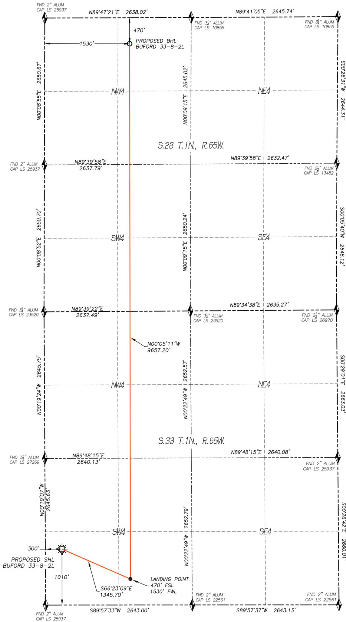
IN ACCORDANCE WITH A REQUEST FROM CONFLUENCE RESOURCES, DALEY LAND SURVEYING, INC. HAS DETERMINED THE SURFACE LOCATION OF THE BUFORD 33-8-2L WELL TO BE 1010' FSL, 300' FWL, AS MEASURED AT NINETY (90) DEGREES FROM THE SECTION LINES OF SECTION 33, TOWNSHIP 1 NORTH, RANGE 65 WEST AND THE BOTTOM HOLE LOCATION TO BE 470' FNL, 1530' FWL, AS MEASURED AT NINETY (90) DEGREES FROM THE SECTION LINES OF SECTION 28, TOWNSHIP 1 NORTH, RANGE 65 WEST, OF THE 6TH PRINCIPAL MERIDIAN, WELD COUNTY, COLORADO.
