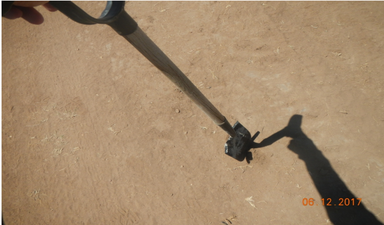
photo 7: The soils at the disturbed area have become heavily compacted. Soil decompaction must occur by cross-ripping to a depth of 18 inches.
