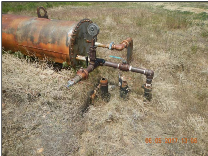
Photo 6. Risers at separator.
