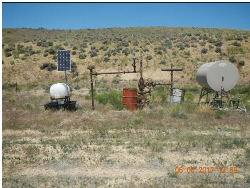
Photo 2. Risers at wellhead. Unlabeled containers adjacent to wellhead.
