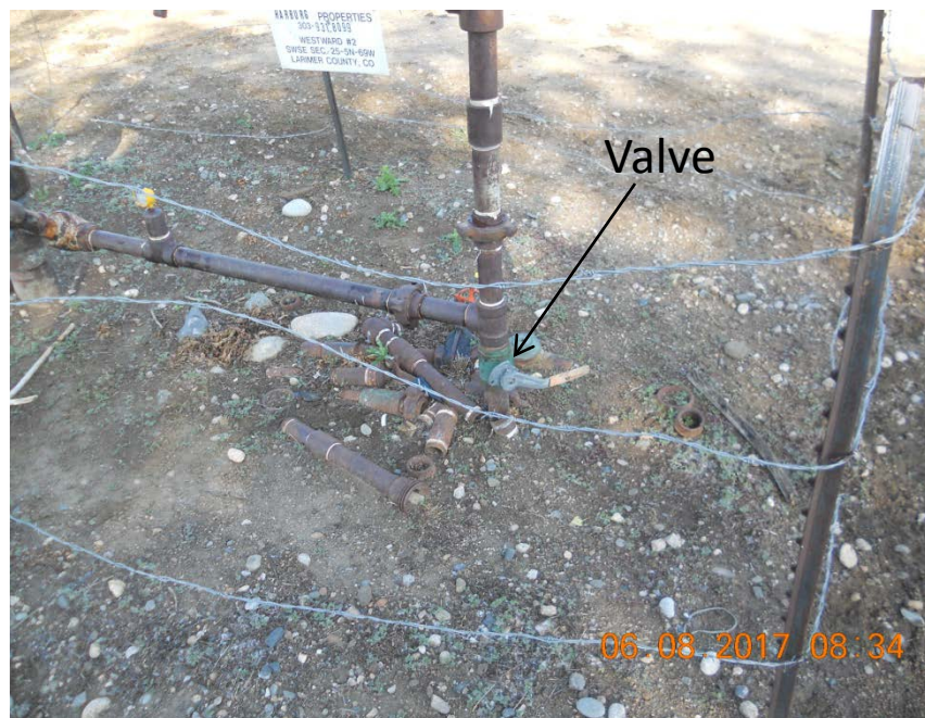
Photo 21. Misc fittings at wellhead. Note closed flowline valve.
