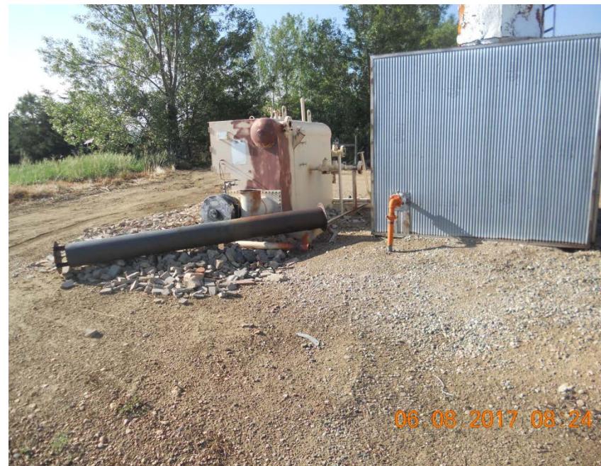
Photo 8. Unused separator at vertical heater treater
