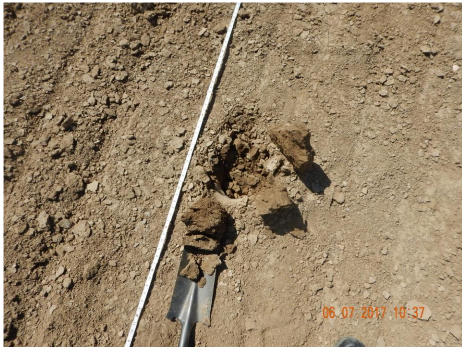
Photo 6: Photo of compaction test pit from the west end of the location. Photo shows compaction layers found in the first 9 inches of soil.
