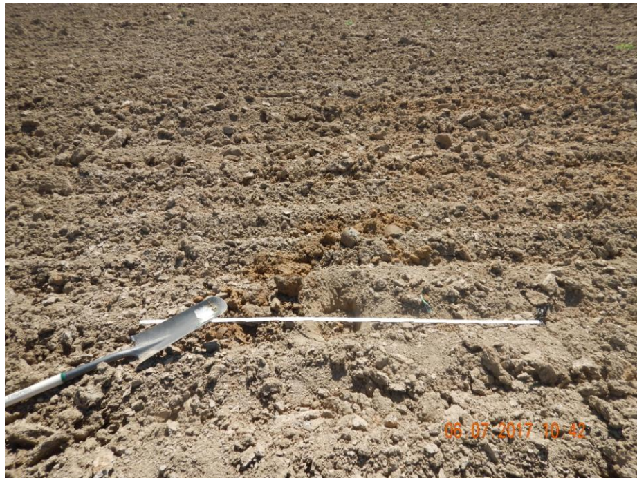
Photo 8: Photo taken from the east end of the location. Photo shows area where a compaction test pit was dug. 6 foot measuring stick for reference.
