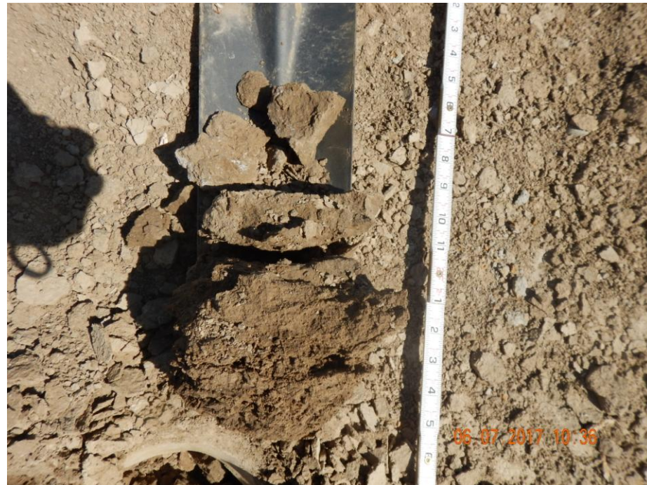
Photo 7: Photo of compaction test pit from the west end of the location. Photo shows compaction layers found in the first 9 inches of soil.
