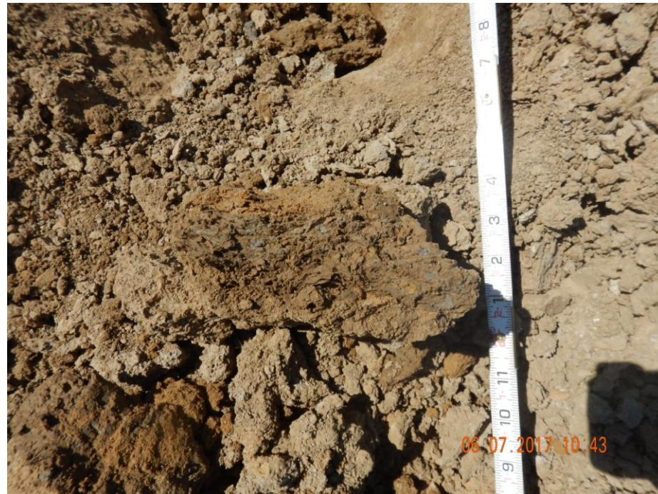
Photo 9: Photo taken from the east end of the location. Photo shows compaction layers found in the first 12 inches.
