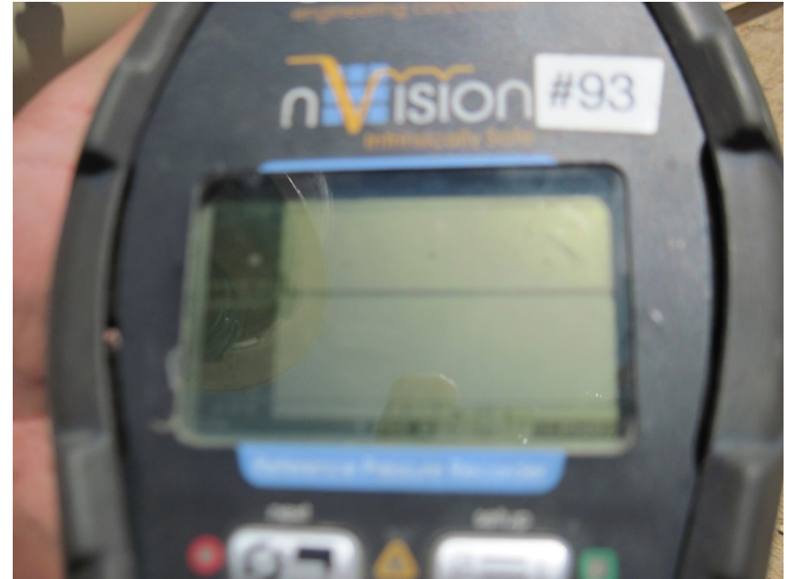
VRU DISCHARGE LINE TESTED GOOD PRESSURE 111 PSI
