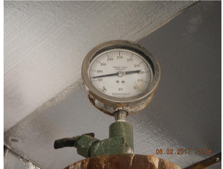
Photo 2 tubing pressure gauge 700 psi
