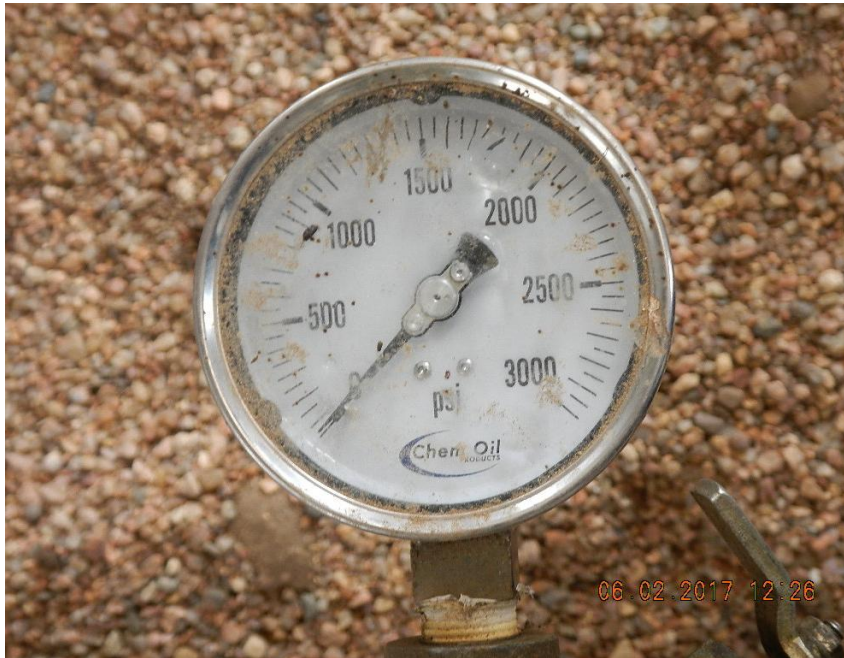
Photo 3 Casing pressure at 0 psi
