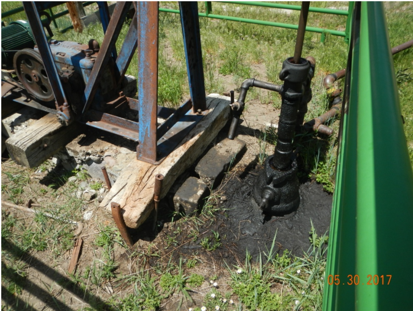
Photo 2. View of discharged oily material appears to be leaking from wellhead.
