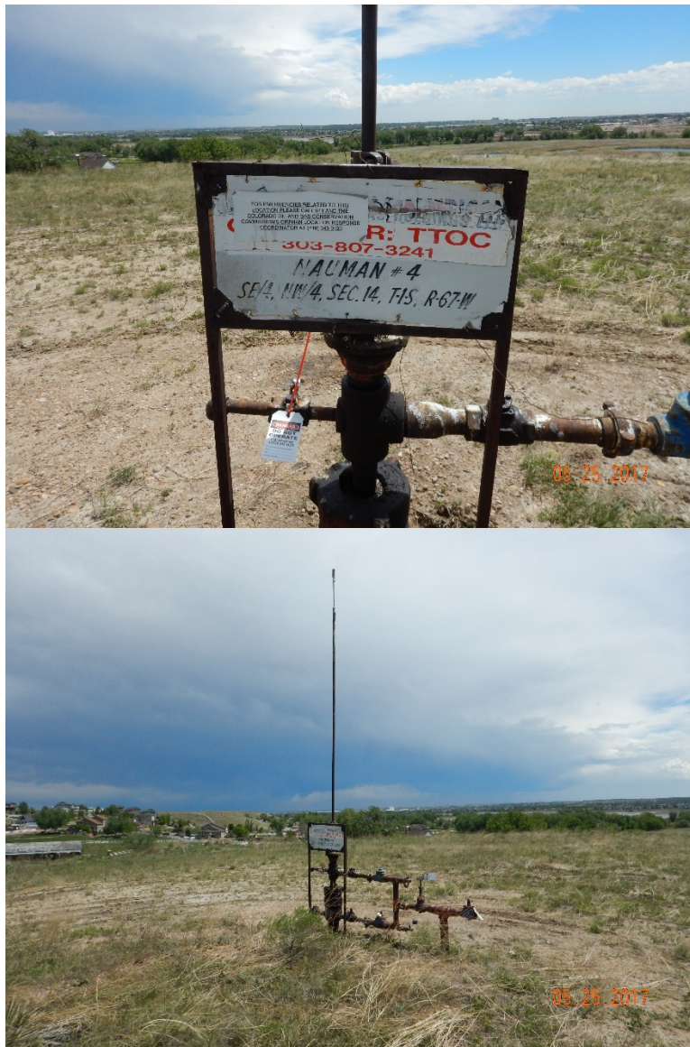
Photos 1 & 2 - Close-up on wellhead sign with COGCC info (top) and photo of wellhead with polished rod (bottom).
