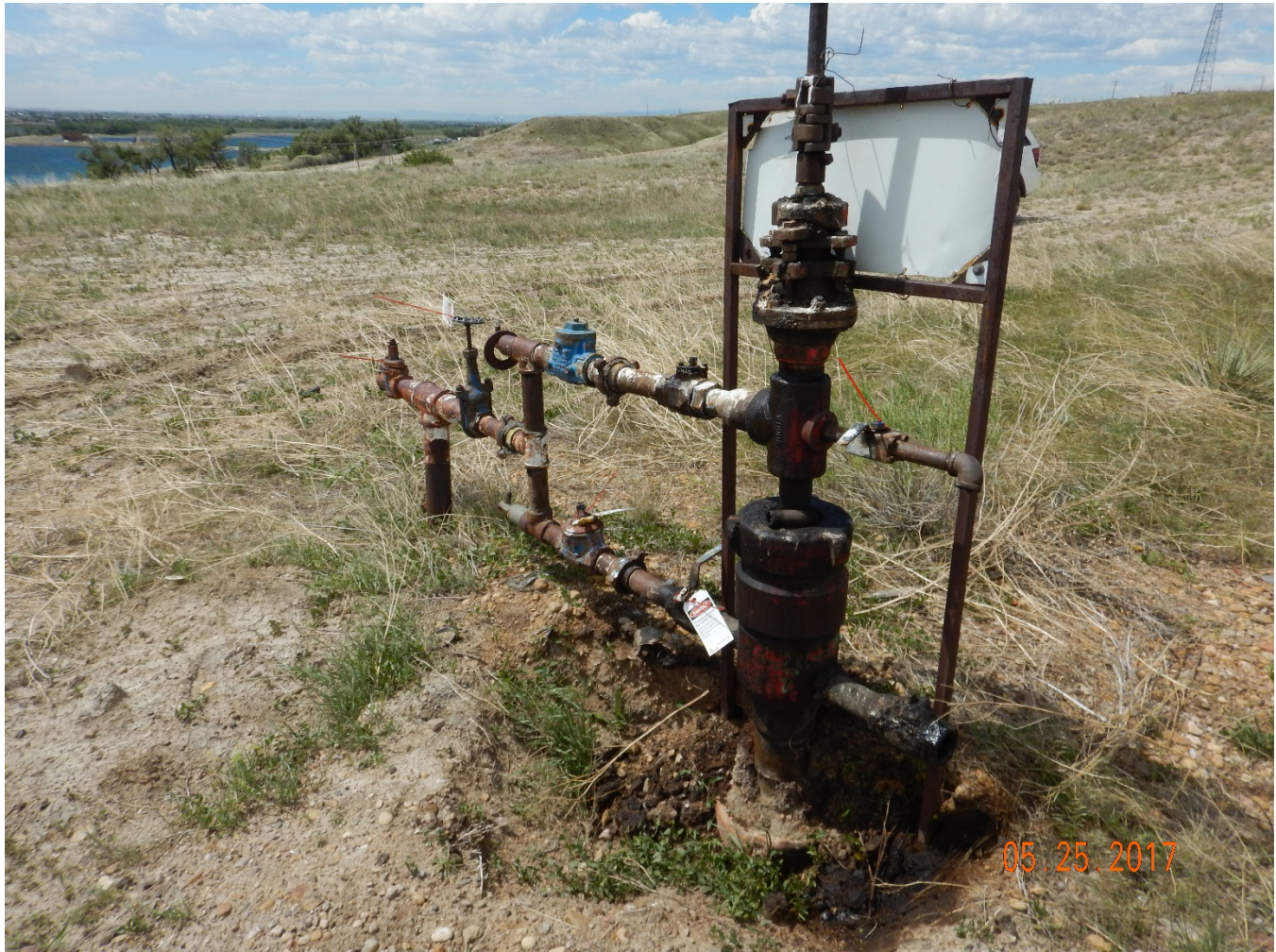
Photo 3 - Close-up on wellhead. Note: COGCC warning tags, localized oil-stained soil, and minor excavation at base of wellhead.
