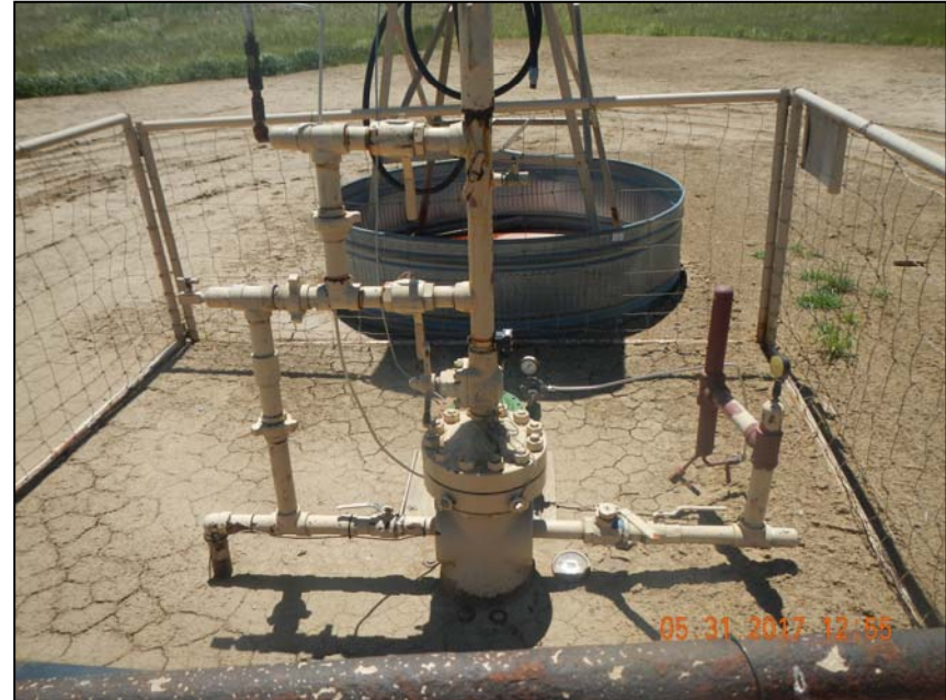
Photo 2. 1 - 2" steel riser at wellhead.
