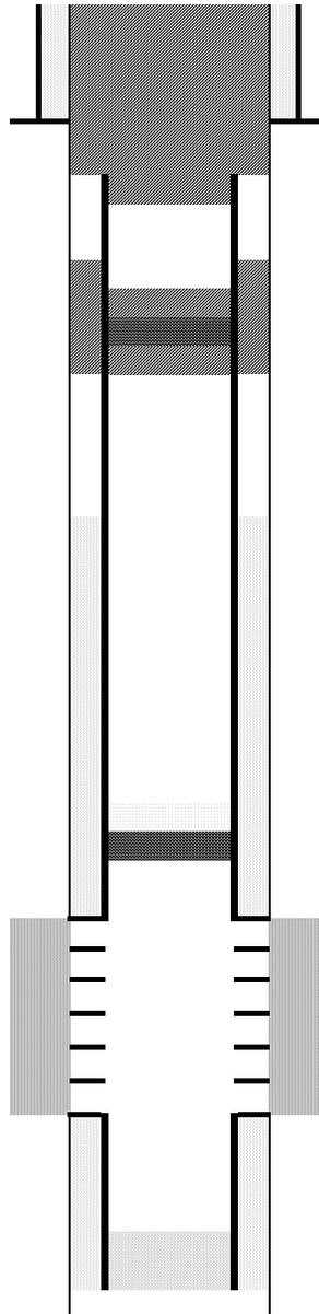
**Cut surface casing off 6'-8' below surface.**
