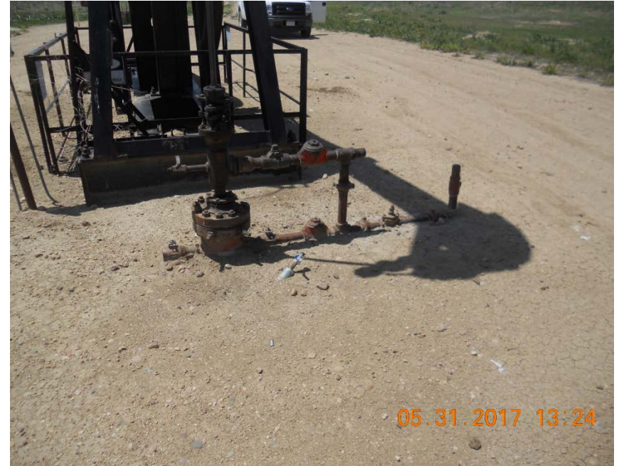
Wellhead and flowline riser
