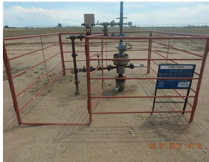
Photo 2: Risers at wellhead
