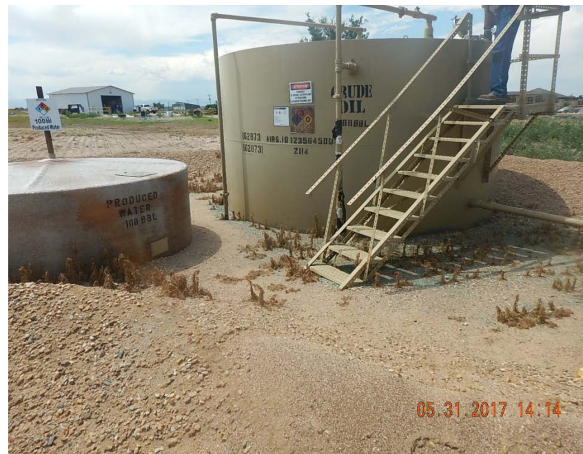
Photo 6: Risers in tank battery
