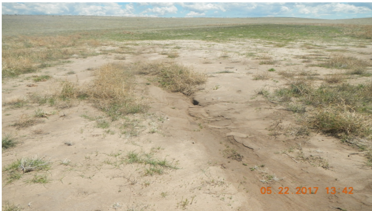
photo 19: Facing toward the south side of the location. There are signs of erosion in this area and inadequate vegetation establishment.
