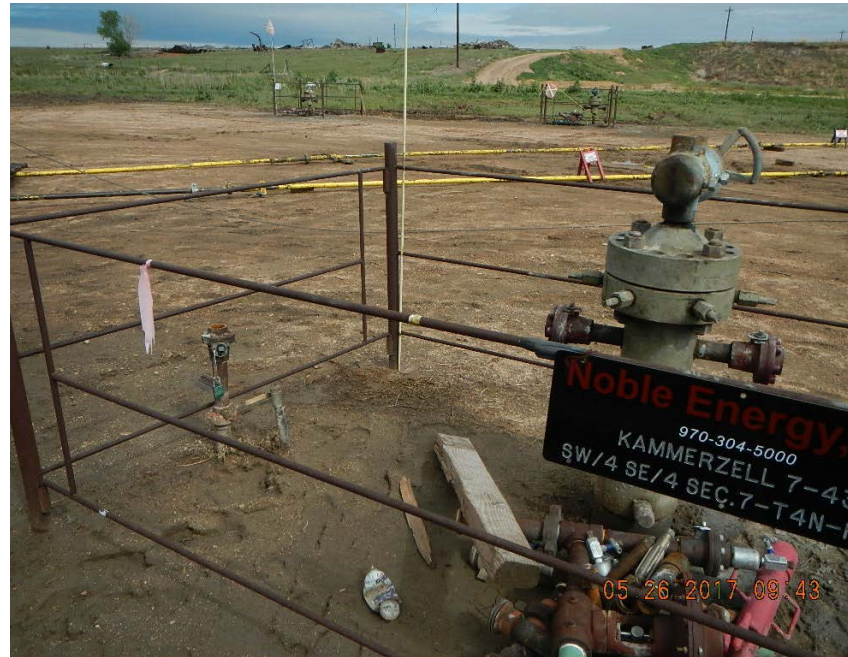
Wellhead and flow lines
