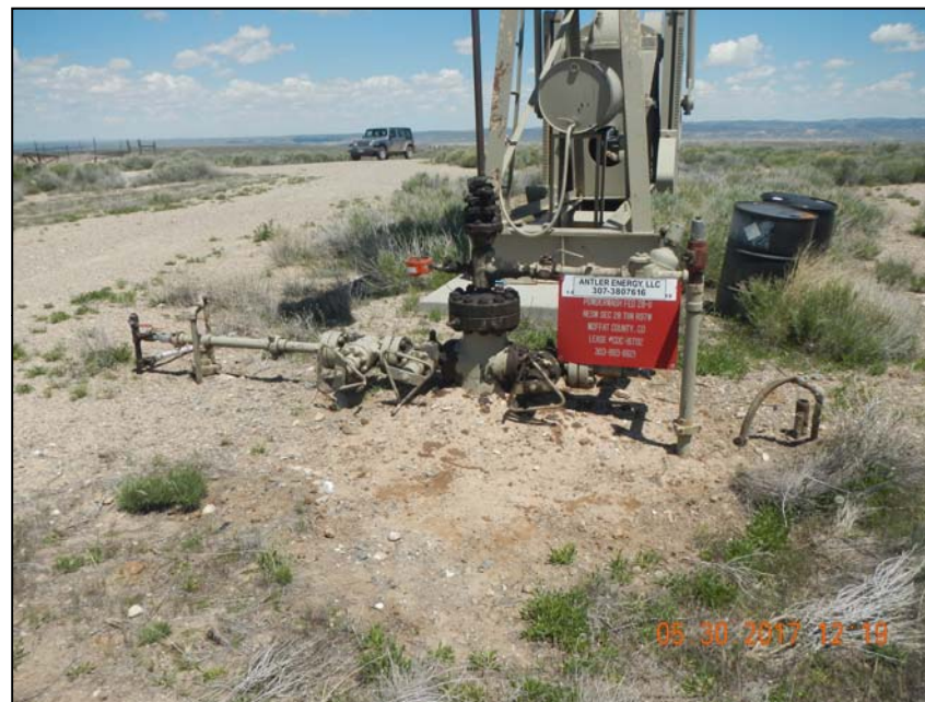
Photo 3. Risers at wellhead. Lube oil containers stored without secondary containment in background.
