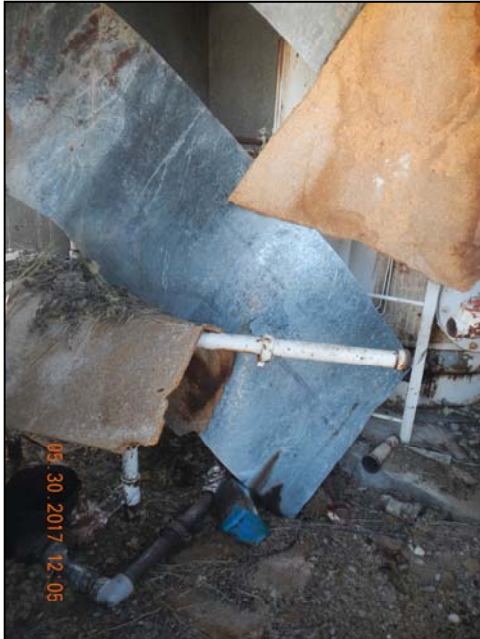
Photo 4. Risers inside stand alone vertical separator.
