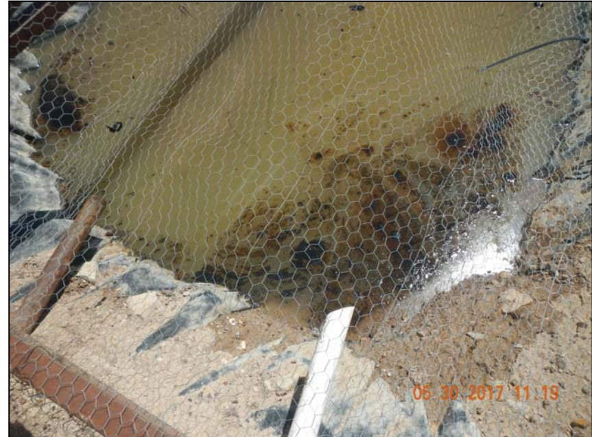
Photo 13. Close-up of flowlines and sheen and oil on pit.
