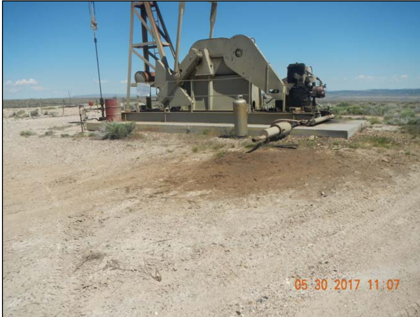
Photo 4. Stained soil at pump jack exhaust.
