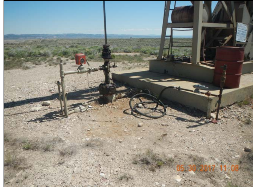
Photo 5. Wellhead. 2 – 1" steel risers, 1 – 2" steel riser, 1 – 2" steel to poly flowline to 1" steel riser.
