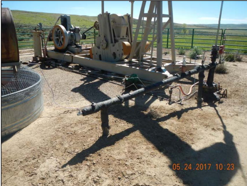
Photo 4. Wellhead assembly showing lines running to separator and motor.
