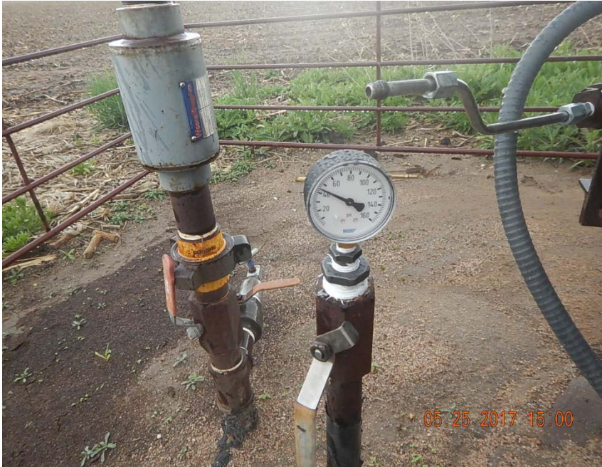
Photo 1: Pressure test at ECD supply line
