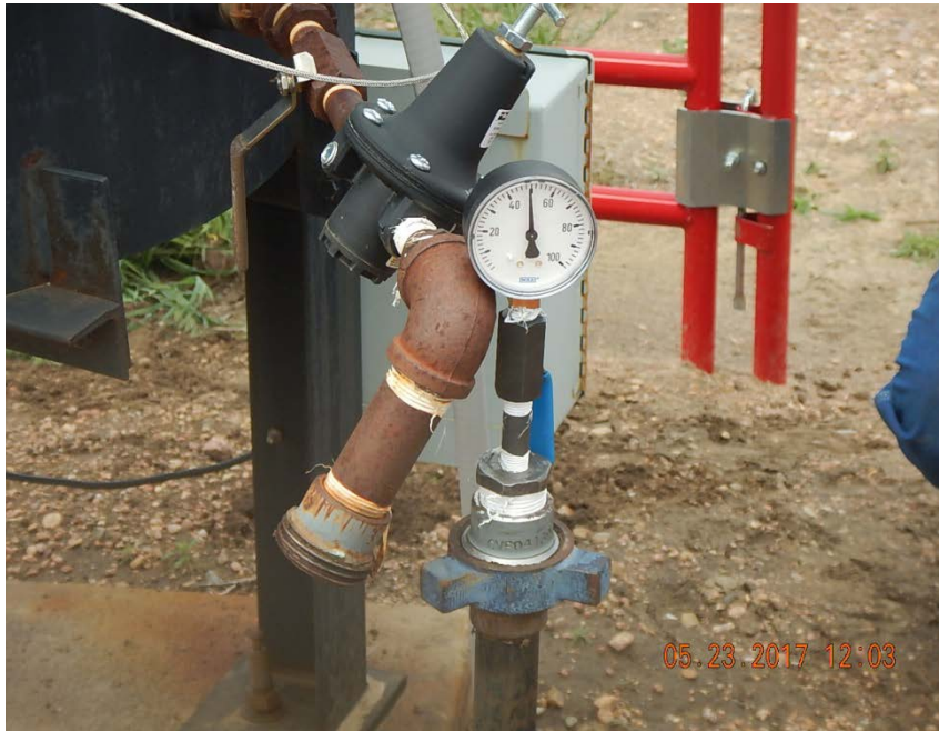
Photo 1: Pressure test on supply line for ECD
