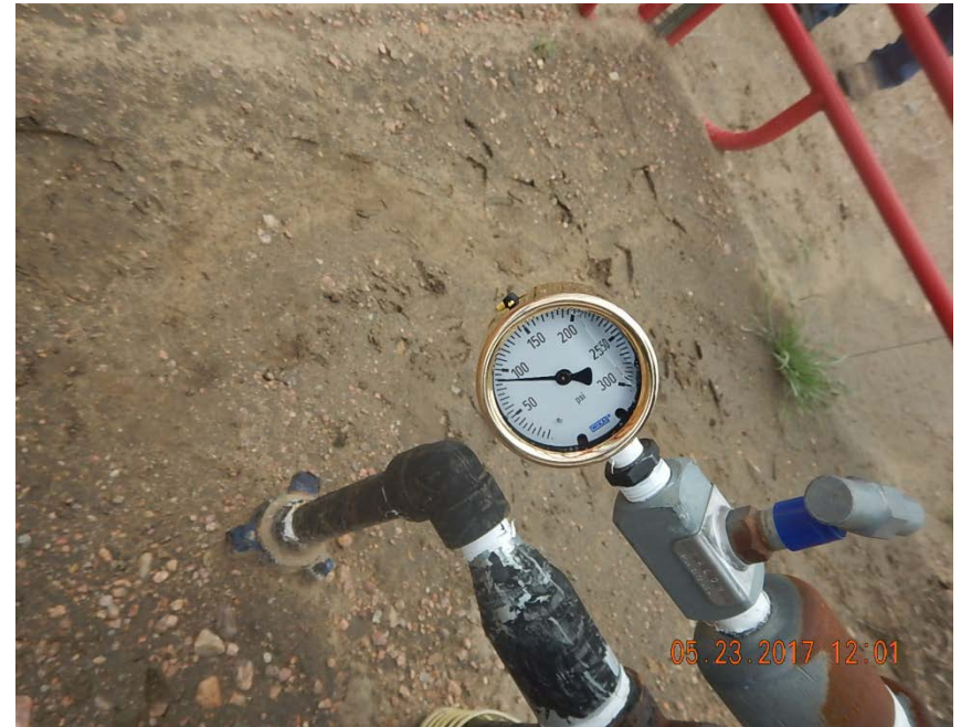
Photo 2: Pressure test for flare line on ECD
