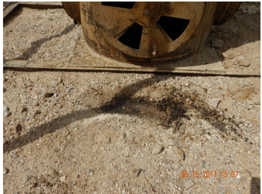
Photo 10. Photo taken on May 15, 2017 from the southeast production area. It appears the impacted soil around the equipment has not been removed. Removal of 1"-2" of gravel on top reveals stained soil with a hydrocarbon like odor.
