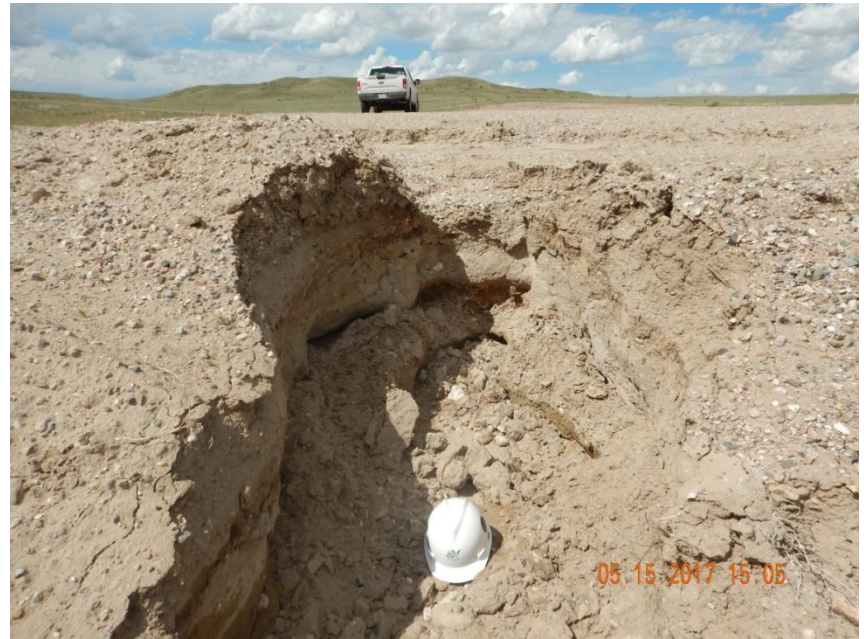
Photo 4. Close-up photo of the gully erosion from the previous photo.
