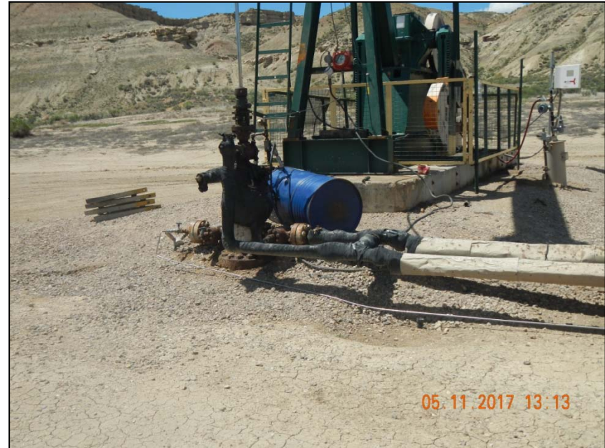
Photo 5. Lube oil at wellhead without secondary containment.
