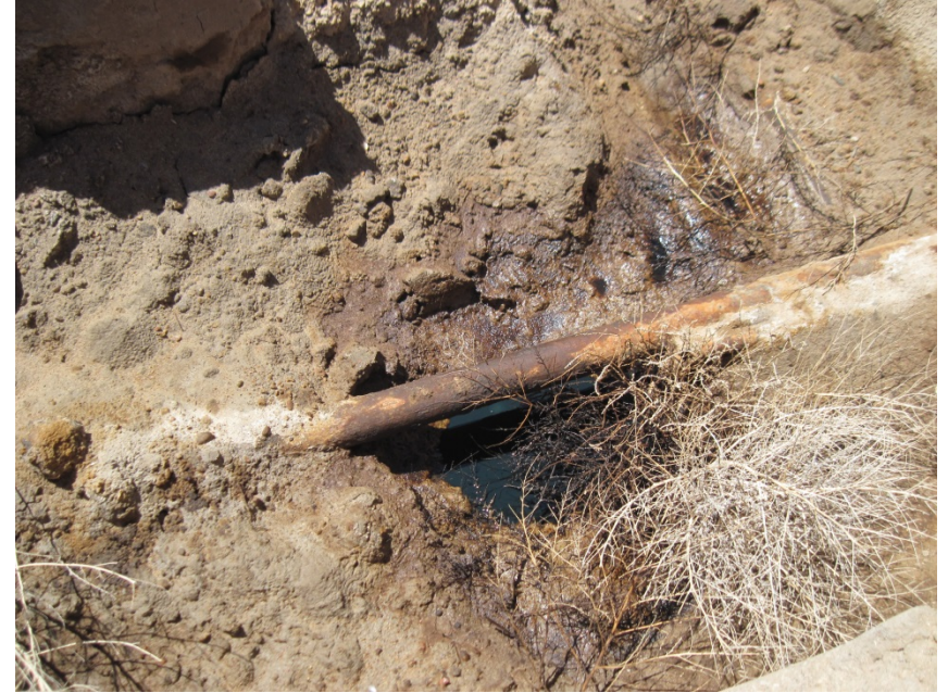
Flow line from Christiansen Unit #2 leaking by Kerr Megee ECD Burner
