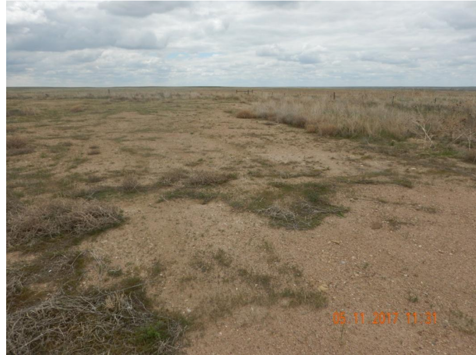
Photo 3: Photo taken from the north end of the Pad well, facing southwest. Photo shows Interim reclamation activities have not been conducted. Gravel/road base remains, location remains predominantly bare and exposed soil. Gravel will need to be removed, area will need to be reclaimed.
