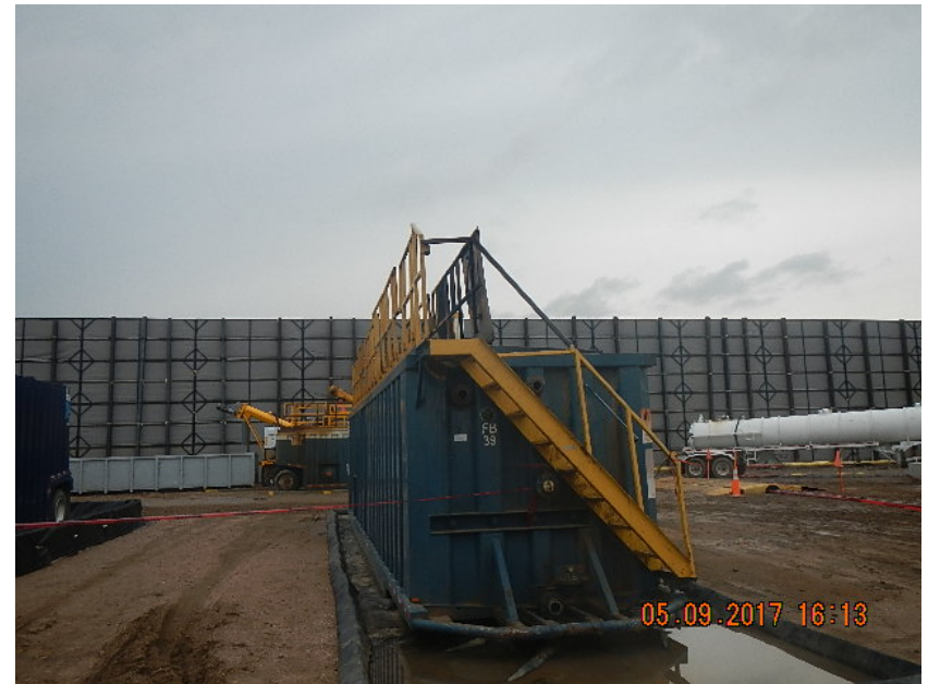
OPEN TOP TANK USED IN FRAC OPERATION AT TIME OF FIRE
